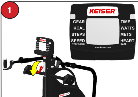
Begin with the computer off and pull Resistance Lever all the way down towards you. This is GEAR "1" position.
