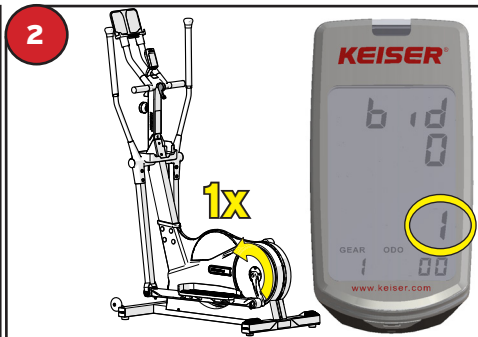
Pedal 1 full revolution to change the TIME value to "1", then stop.
